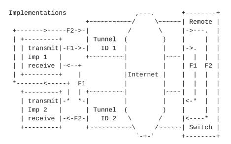
Illustrations of a test setup with a bi-directional tunnel. The upper diagram emphasizes the VLAN connectivity and geographical location (where "Imp #" is the sender and receiver of implementation 1 or 2, either Perfas+ and NetProbe in this test). The lower diagram shows example flows traveling between two measurement implementations. For simplicity only two flows are shown, and netem is omitted (it would appear before or after the Internet, depending on the flow).
