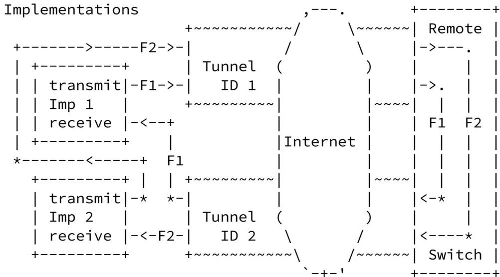
Illustrations of a test setup with a bi-directional tunnel. The upper diagram emphasizes the VLAN connectivity and geographical location (where "Imp #" is the sender and receiver of implementation 1 or 2, either Perfas+ and NetProbe in this test). The lower diagram shows example flows traveling between two measurement implementations. For simplicity only two flows are shown, and netem is omitted (it would appear before or after the Internet, depending on the flow).
