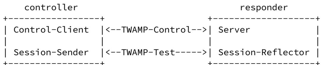
This example provides an architecture that supports the full TWAMP standard. The controller establishes the test session with the responder through the TWAMP-Control protocol. After the session is established the controller transmits test packets to the responder. The responder follows the Session-Reflector behavior of TWAMP as described in [section 4.2](#).
