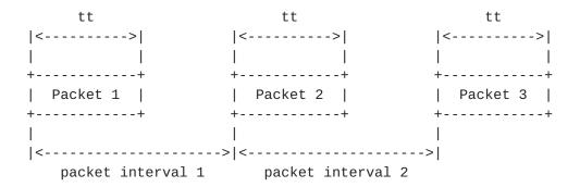
The test packet size and interval between consecutive packets for each train sent by the Session-Sender and reflected by the Session-Reflector MUST be calculated and determined by the controller or an application or entity communicating with the controller. The packet size and interval MAY vary within a train and/or between trains. Determination of the packet size and interval is implementationspecific.
