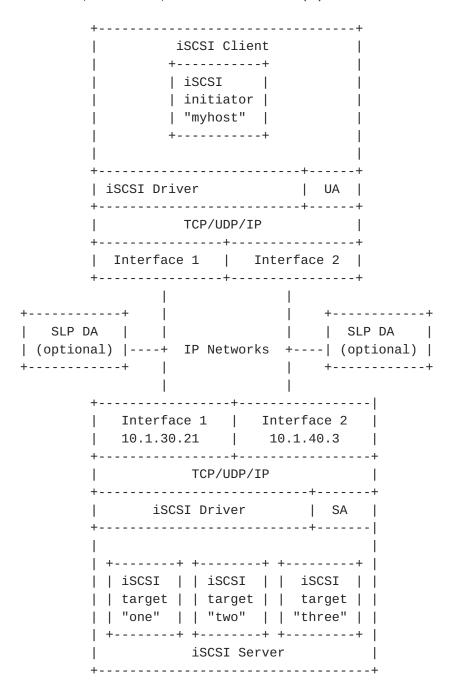
In the above drawing, the iSCSI server has three iSCSI targets that the client could discover, named "one", "two" and "three". The iSCSI client has an iSCSI initiator with the name "myhost". The iSCSI client may use the initiator name in its SLP Service Requests as a filter to discover only targets that are configured to accept iSCSI connections from "myhost".
