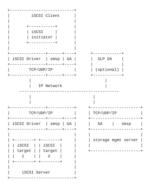
Note the difference between the storage management server model and the previously-defined target discovery model. When target discovery was used, the iSCSI Server implemented an SA, to be discovered by the initiator's UA. In the storage management server model, the iSCSI clients and servers both implement UAs, and the management server implements the SA.
