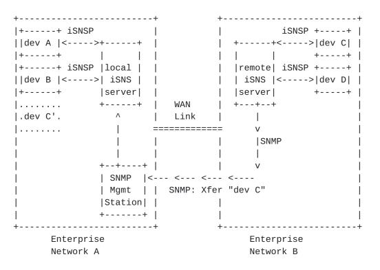
The above diagram illustrates a second example of how iSNS records can be shared. This method uses an SNMP-based management station to (manually) retrieve (GET) the desired record for "dev C", and then directly store (SET) it on the local iSNS server. Once the record is transferred to the local iSNS server in Network A, "dev C" becomes visible and accessible (provided firewall boundaries can be negotiated) to other devices in Network A.
