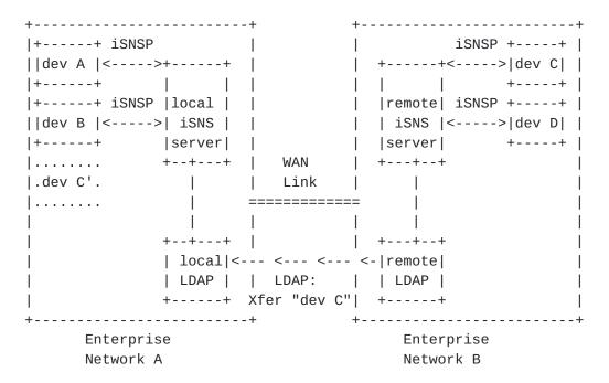
In the above diagram, two business partners wish to share storage "dev C". Using LDAP, the record for "dev C" can be transferred from Network B to Network A. Once accessible to the local iSNS server in Network A, local devices A and B can now discover and connect to "dev C".
