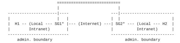
Only tunnel mode is required here. So the headers in a packet between SG1 and SG2 could look like either of the following:
