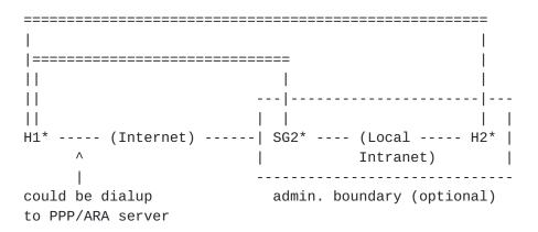
Only tunnel mode is required between H1 and SG2. So the choices for the SA between H1 and SG2 would be one of the ones in case 2. The choices for the SA between H1 and H2 would be one of the ones in case 1.
