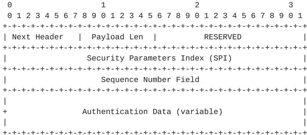
The following subsections define the fields that comprise the AH format. All the fields described here are mandatory, i.e., they are always present in the AH format and are included in the Integrity Check Value (ICV) computation (see Sections 2.6 and 3.3.3).
