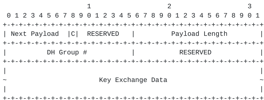
Figure 10: Key Exchange Payload Format
