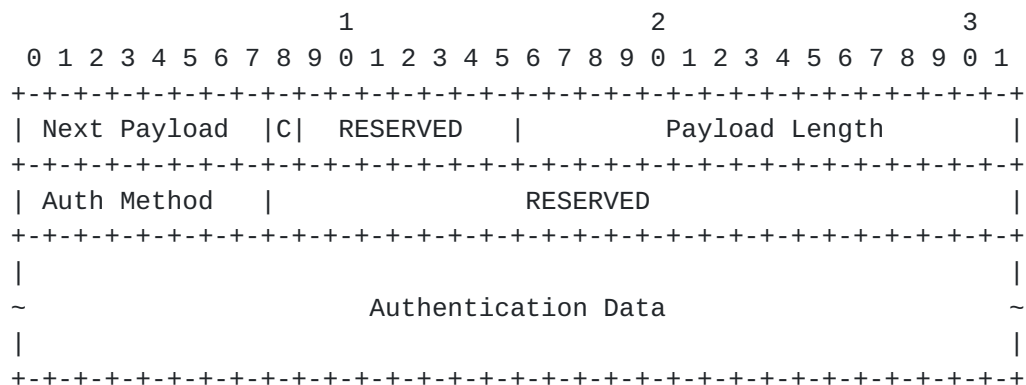
Figure 14: Authentication Payload Format
