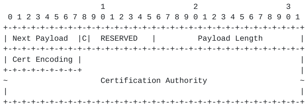
Figure 13: Certificate Request Payload Format
