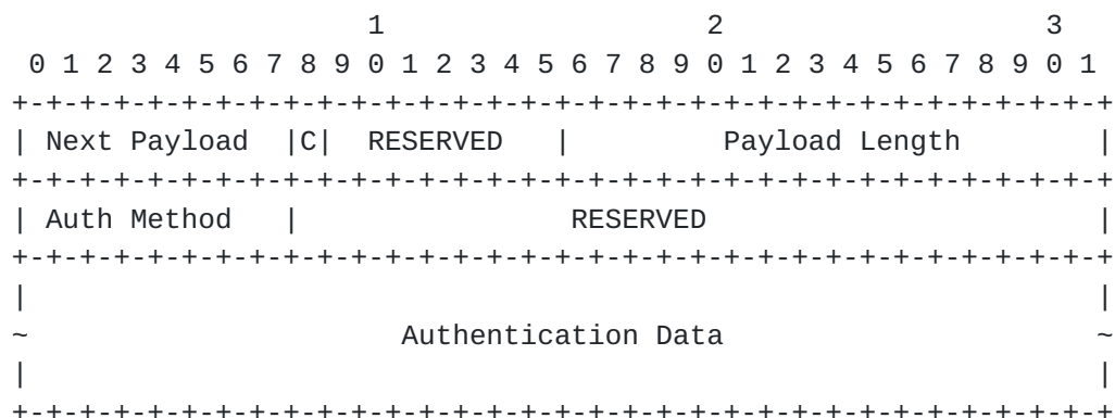
Figure 14: Authentication Payload Format
