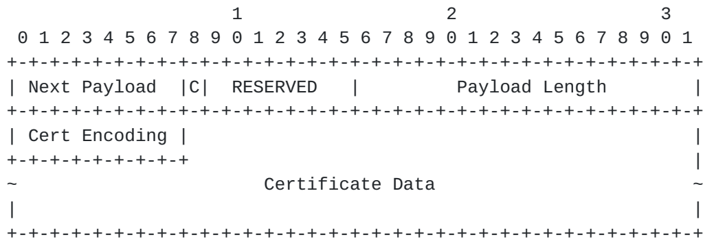
Figure 12: Certificate Payload Format
