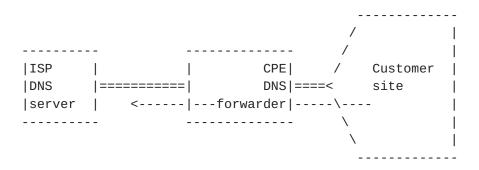
In this configuration, the CPE is acting as a multi-sited router.
