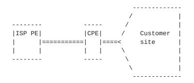
The customer router CPE could be configured on its internal interface with one of the reserved site local addresses and listen for DNS queries. It would be configured to use one (or several) of the well known site local unicast addresses within the ISP's site to send its own queries to. It would act as a DNS forwarder, forwarding queries received on its internal interface to the ISP's recursive DNS server.
