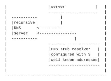
(The recursive DNS server is configured to listen both on its IPv6 address and on the well known address)
