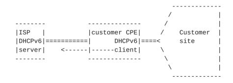
This example will show how DHCPv6 and well known site local unicast addresses cooperate to enable the internal nodes to access DNS.
