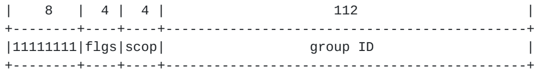
Figure 1: Generic IPv6 multicast address format
