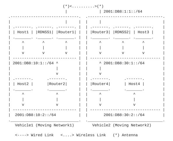
Figure 3: Internetworking between Two Vehicle Networks
