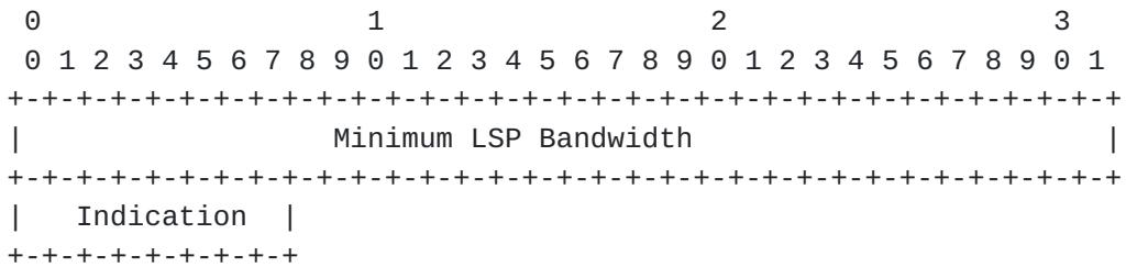
The Minimum LSP Bandwidth is encoded in a 4 octets field in the IEEE floating point format. The units are bytes (not bits!) per second. The indication whether the interface supports Standard or Arbitrary SONET/SDH is encoded as 1 octet. The value of this octet is 0 if the interface supports Standard SONET/SDH, and 1 if the interface supports Arbitrary SONET/SDH.
