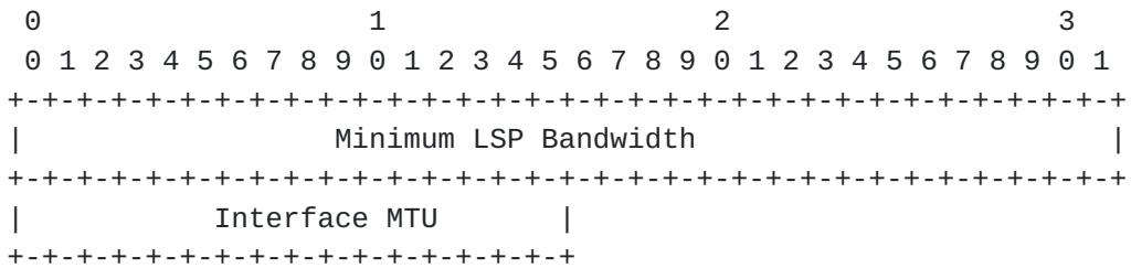
The Minimum LSP Bandwidth is encoded in a 4 octets field in the IEEE floating point format. The units are bytes (not bits!) per second. The Interface MTU is encoded as a 2 octets integer.
