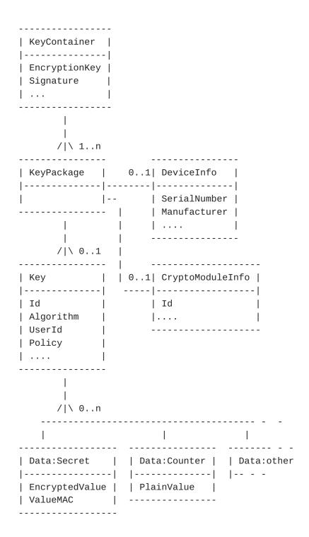
Figure 1: PSKC data elements relationship diagram
