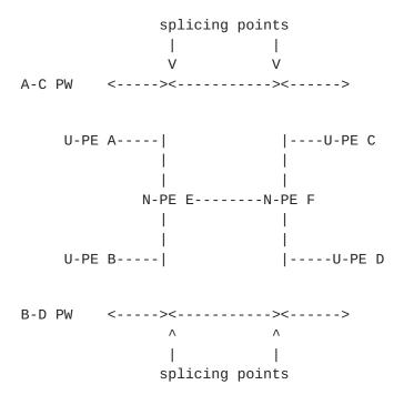
One can see that distributed VPLS does not reduce the number of pseudowires per U-PE, but it does reduce the number of control connections per U-PE. Whether this is worthwhile depends, of course, on what the bottleneck is.
