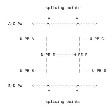
One can see that distributed VPLS does not reduce the number of pseudowires per U-PE, but it does reduce the number of control connections per U-PE. Whether this is worthwhile depends, of course, on what the bottleneck is.
