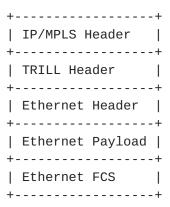
Figure 3: TRILL over MPLS Encapsulation
