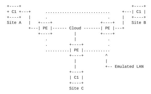
The set of PE devices interconnected via pseudowires appears as a single emulated LAN to customer C1. Each PE device will learn remote MAC address to pseudowire associations and will also learn directly attached MAC addresses on customer facing ports.
