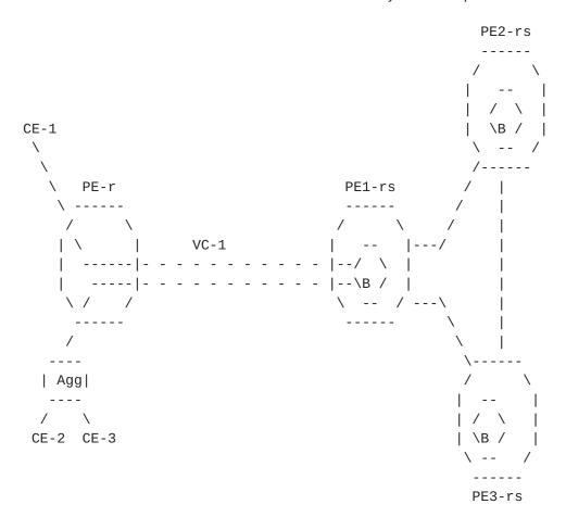
to participate in a VPLS service, the PE-r device creates a pointto-point [PWE3-ETHERNET] pseudowire that terminates on the physical port at the PE-r and terminates on the virtual bridge instance of the VPLS service at the PE-rs.
