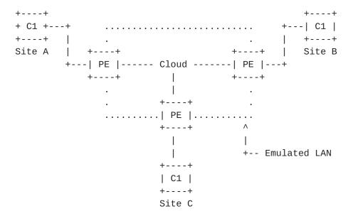
The set of PE devices interconnected via pseudowires appears as a single emulated LAN to customer C1. Each PE device will learn remote MAC address to pseudowire associations and will also learn directly attached MAC addresses on customer facing ports.
