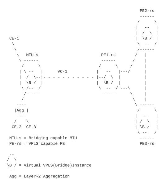
The MTU-s device and the PE-rs device treat each spoke connection like an access port of the VPLS service. On access ports, the combination of the physical port and/or the VLAN tag is used to associate the traffic to a VPLS instance while the pseudowire tag (e.g., VC label) is used to associate the traffic from the virtual spoke port with a VPLS instance, followed by a standard L2 lookup to identify which customer port the frame needs to be sent to.
