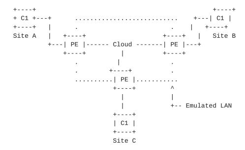
The set of PE devices interconnected via PWs appears as a single emulated LAN to customer C1. Each PE device will learn remote MAC address to PW associations and will also learn directly attached MAC addresses on customer facing ports.
