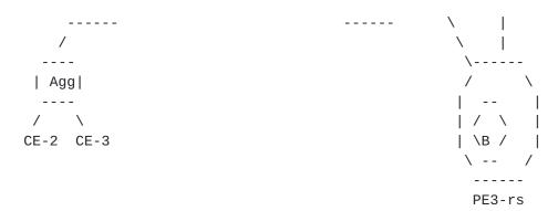
Then for every access port that needs to participate in a VPLS service, the PE-r device creates a point-to-point [PWE3-ETHERNET] PW that terminates on the physical port at the PE-r and terminates on the virtual bridge instance of the VPLS service at the PE-rs.
