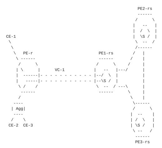
Then for every access port that needs to participate in a VPLS service, the PE-r creates a point-to-point PW that terminates on the physical port at the PE-r and terminates on the VSI of the VPLS service at the PE-rs.
