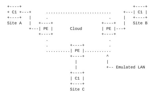
We note here again that while this document shows specific examples using MPLS transport tunnels, other tunnels that can be used by PWs (as mentioned in [PWE-CTRL]), e.g., GRE, L2TP, IPSEC, etc., can also be used, as long as the originating PE can be identified, since this is used in the MAC learning process.
