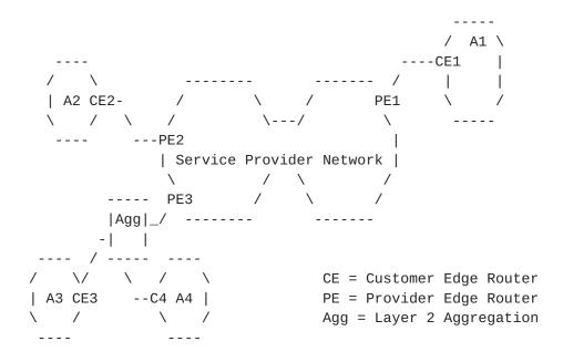
Initially, the VPLS is set up so that PE1, PE2 and PE3 have a full mesh of Ethernet PWs. The VPLS instance is assigned a identifier
