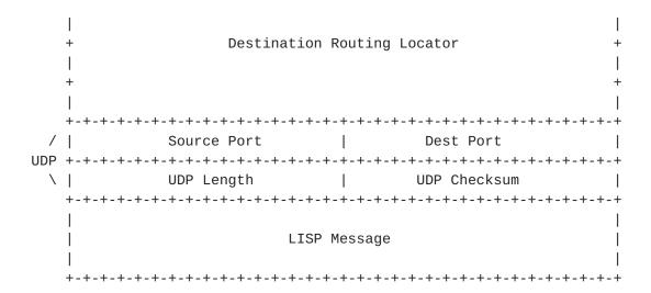
The LISP UDP-based messages are the Map-Request and Map-Reply messages. When a UDP Map-Request is sent, the UDP source port is chosen by the sender and the destination UDP port number is set to 4342. When a UDP Map-Reply is sent, the source UDP port number is set to 4342 and the destination UDP port number is copied from the source port of either the Map-Request or the invoking data packet.
