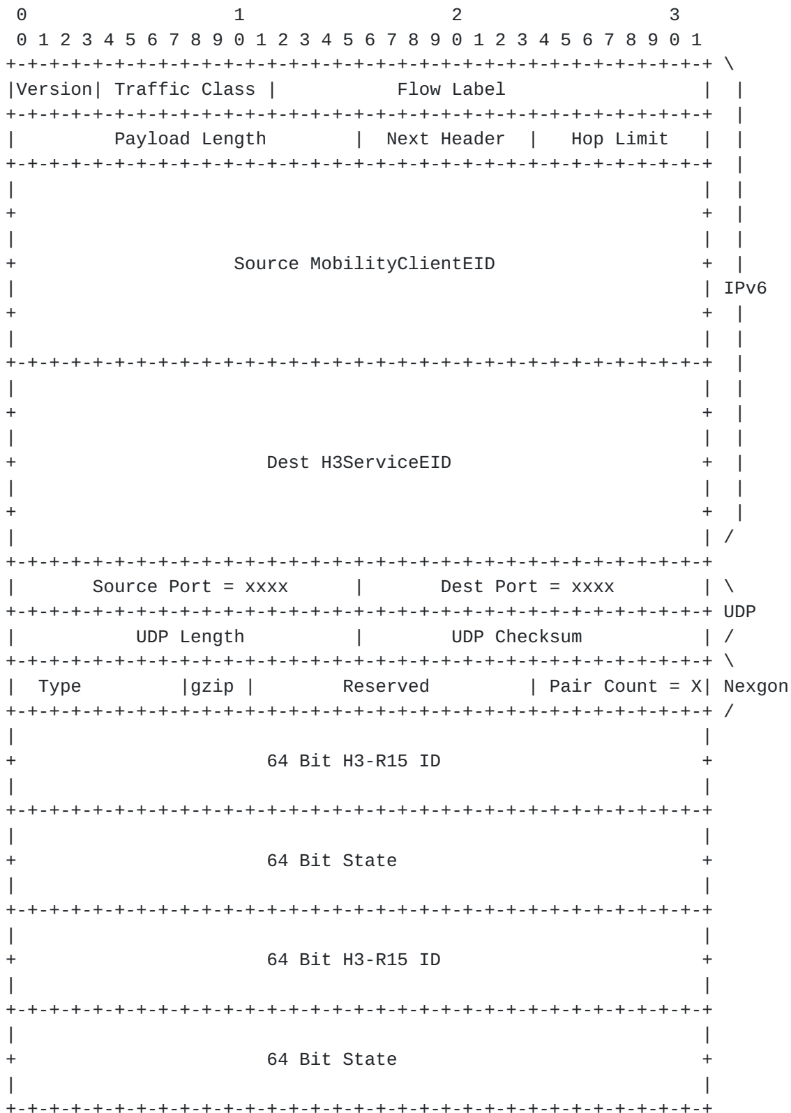
Figure 6: Published detections packet format
