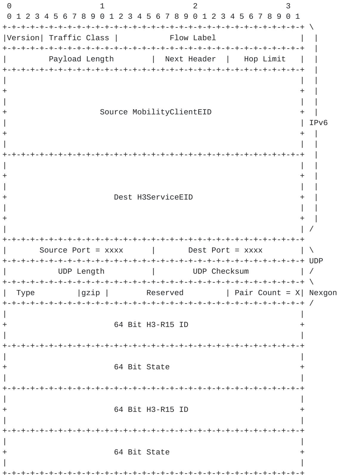
Figure 6: Uploaded detections packet format
