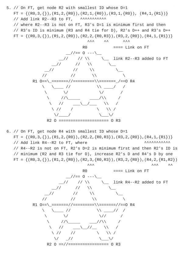
FT is computed, which has Degree of 3 and Diameter of 2.
