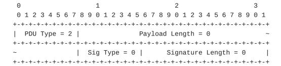
L3DL devices SHOULD beacon frequent Layer-2 KEEPALIVE PDUs to ensure session continuity. The inter-KEEPALIVE interval is configurable, with a default of ten seconds. A receiver may choose to ignore KEEPALIVE PDUs.
