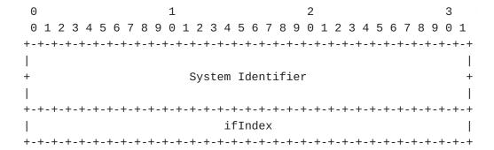
System Identifier, a la [RFC1629], is an eight octet identifier unique in the entire operational space. Routers and switches usually have internal MAC Addresses which can be padded with high order zeros and used if no System ID exists on the device. If no unique identifier is burned into a device, the local L3DL configuration SHOULD create and assign a unique one, likely by configuration.
