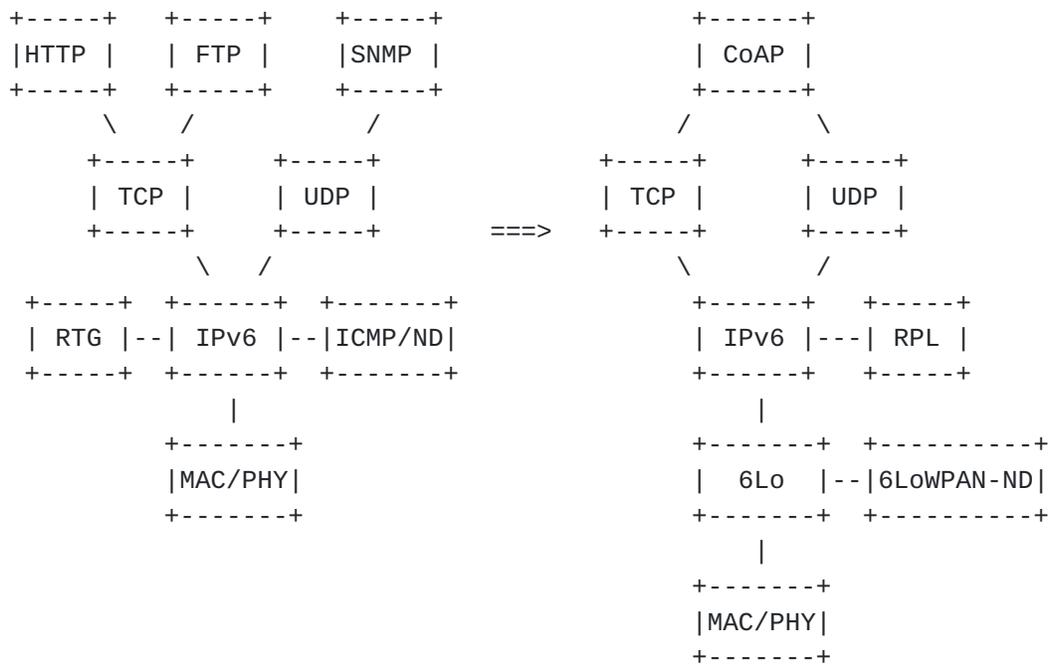
Figure 1: Traditional and Light-weight Internet Protocol Stack
