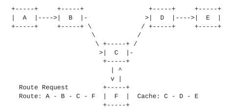
The concatenation of the accumulated route record from the Route Request and the cached route from F's Route Cache would include a duplicate node in passing from C to F and back to C.
