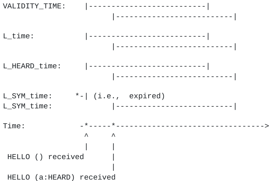
Figure 7: HELLO message processing: network address present
