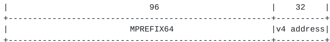
Figure 2: IPv4-Embedded IPv6 Multicast Address Format
