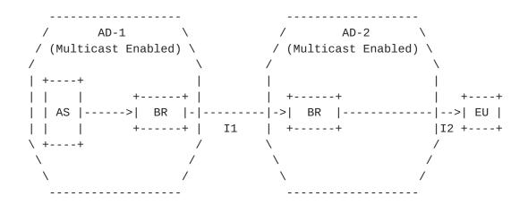
AD = Administrative Domain (Independent Autonomous System) AS = Application (e.g., Content) Multicast Source BR = Border Router I1 = AD-1 and AD-2 Multicast Interconnection (e.g., MBGP) I2 = AD-2 and EU Multicast Connection
