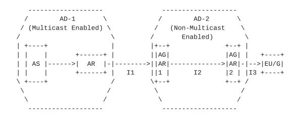
AS = Application Source AR = AMT Relay in AD-1AGAR1 = AMT Gateway/Relay node in AD-2 across Peering Point II = AMT Tunnel Connecting AR in AD-1 to GW in AGAR1 in AD-2 AGAR2 = AMT Gateway/Relay node at AD-2 Network Edge I2 = AMT Tunnel Connecting Relay in AGAR1 to GW in AGAR2 EU/G = Gateway client embedded in EU device I3 = AMT Tunnel Connecting EU/G to AR in AGAR2
