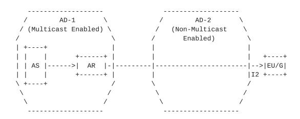
AS = Application Multicast Source AR = AMT Relay EU/G = Gateway client embedded in EU device I2 = AMT Tunnel Connecting EU/G to AR in AD-1 through Non-Multicast Enabled AD-2.
