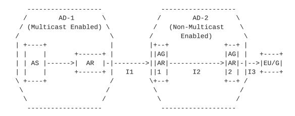
AS = Application Source AR = AMT Relay in AD-1AGAR1 = AMT Gateway/Relay node in AD-2 across Peering Point I1 = AMT Tunnel Connecting AR in AD-1 to GW in AGAR1 in AD-2 AGAR2 = AMT Gateway/Relay node at AD-2 Network Edge I2 = AMT Tunnel Connecting Relay in AGAR1 to GW in AGAR2 EU/G = Gateway client embedded in EU device I3 = AMT Tunnel Connecting EU/G to AR in AGAR2
