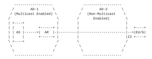
AS = Application Multicast Source AR = AMT Relay EU/G = Gateway client embedded in EU device I2 = AMT Tunnel Connecting EU/G to AR in AD-1 through Non-Multicast Enabled AD-2.
