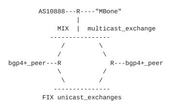
AS10888 acts as a transit AS to connect other multicast-friendly exchanges to the NASA ARC MIX. It also acts as a gateway between the DVMRP-based "Mbone" and the BGP4+ area.
