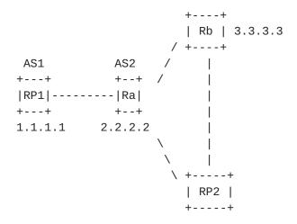
Where RP2 MSDP and MBGP peers with Ra (using 2.2.2.2) and with Rb (using 3.3.3.3). When the MSDP SA update arrives on RP2 from Ra, the MSDP RPF check for 1.1.1.1 passes because RP2 receives the SA update from MSDP peer 2.2.2.2 which is also the correct MBGP next hop for 1.1.1.1.
