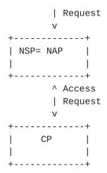
In this case the NSP is the sole entity providing Network Service Provision including Network Access Provision to the User. First a user that requests content sends an Access request to an NSP which then forwards it on to the appropriate CP for Authentication and Authorization purposes. The CP responds with either "success" or "failure". If "success", the NSP may forward a success response and stream multicast data to the user.
