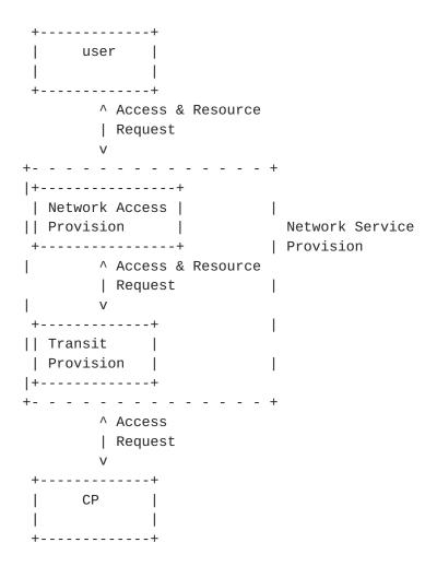
For the sake of simplification the above diagram shows a 1-1 relationship between an NAP and a TP. However it is also possible for a single NAP to connect to multiple TPs, and a single TP to multiple NAPs.
