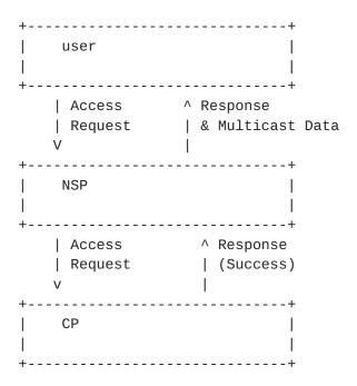
For the sake of simplicity, the above diagram portrays a case where there is a single NSP entity and a single CP entity, but multiple CPs can be connected to the same NSP. It is also possible for the same CP to be connected to multiple NSP networks (e.g. network selection). In other words the relationship of NSP:CP can be described as 1:1, 1:N or M:N. Furthermore it is possible that the NSP and CP could be the same entity.
