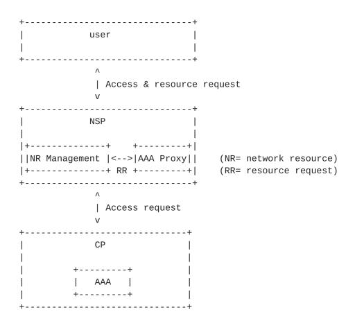
In the fully enabled model the NSP provides proxying of authentication and authorization between the NSP and CP, as well as user-based accounting. The AAA proxy server of the NSP communicates with the CP's AAA server. Although not shown in the above diagram for the sake of simplicity, in addition to direct proxying between a NSP and CP, this proxying may be done through a TP. This means that the transit provider is also cable of supporting AAA proxying.
