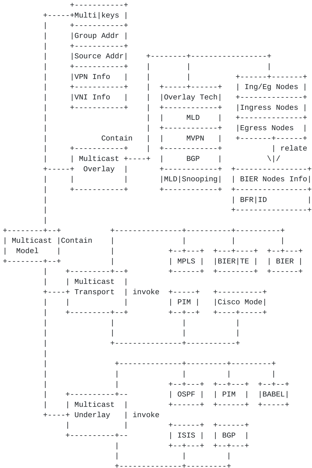
Figure 3: UML like Class Diagram for Multicast YANG data Model
