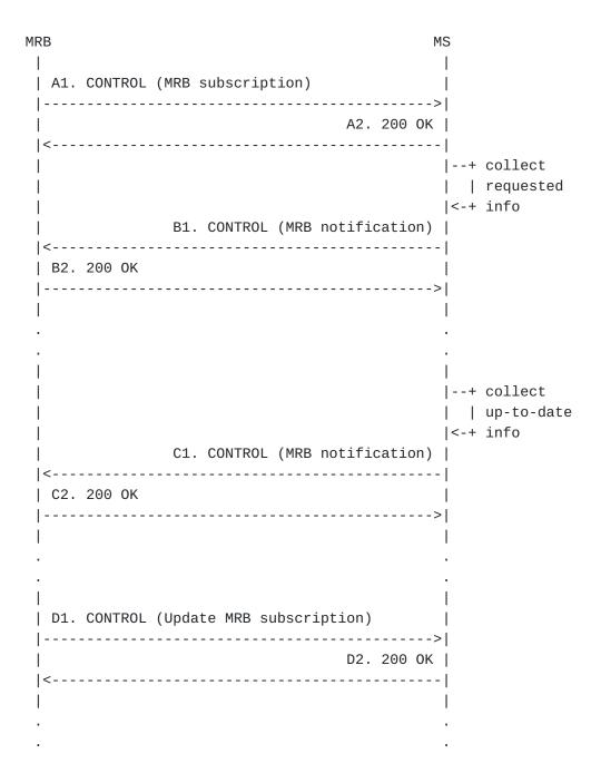
In this example, the MRB subscribes for information at the specified MS, and events are triggered at a regular, negotiated, basis. All this messages flow through the control channel as all the messages in this document. The framework transaction steps are the following:
