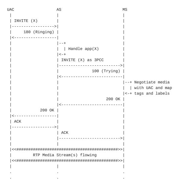
Note well: this is only an example of a possible approach involving a 3PCC negotiation among the UAC, the AS and the MS, and as such is not at all to be considered as the mandatory way or as best common practice either in the presented scenario. [RFC3725] provides several different solutions and many details about how 3PCC can be realized, with pros and cons.
