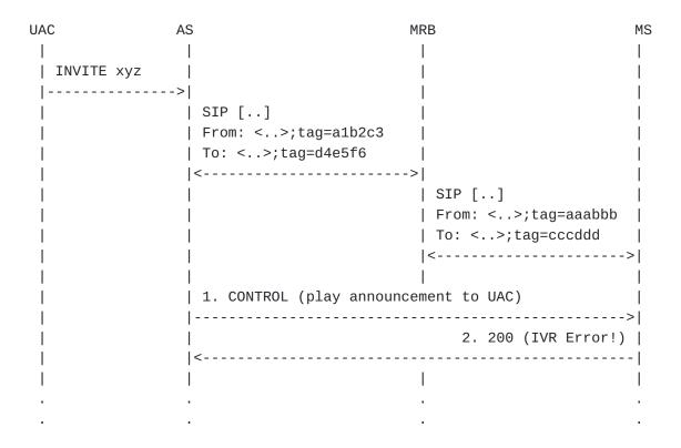
In the example, once done with the 3PCC and the UAC being attached to the MS, the AS and the MS end up with different assumptions with respect to the 'connectionid' addressing UAC. In fact, the AS builds a 'connectionid' using the tags it is aware of (a1b2c3:d4e5f6), while the
