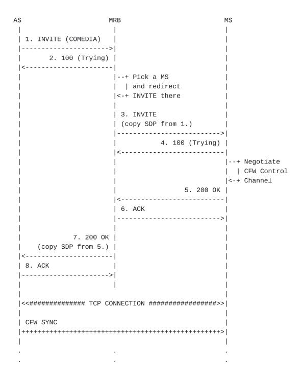
As it can be evinced from the diagram, in this topology the MRB basically acts as a 3PCC between the AS and the chosen MS. The same can be said with respect to attaching UAC call legs. The MRB remembers the MS it has chosen for the AS and, for every UAC call leg the AS tries to attach to the MRB, it makes sure it is actually redirected to the MS somehow.
