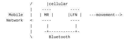
The camera (Local Fixed Node) uploads photographic content to a Correspondent Node (CN) server. When the mobile network moves away, the Mobile Router serving the mobile network changes its point of attachment from one cellular access (Access Router) to another, obtaining a new Care-of Address. The Home Agent (HA) encapsulates application traffic for CN and LFN.
