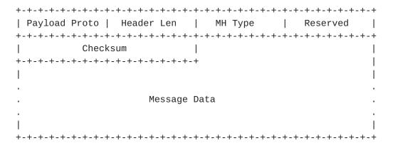
See <a href="RFC 3775">RFC 3775</a> [2] for a description of the 'Payload Proto', 'Header Len', 'MH Type', 'Reserved' and the 'Checksum' fields.
