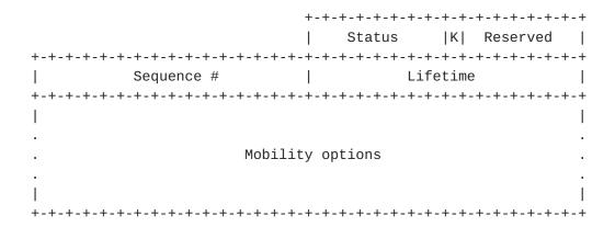
Figure 9: Fast Binding Acknowledgment (FBack) Message
