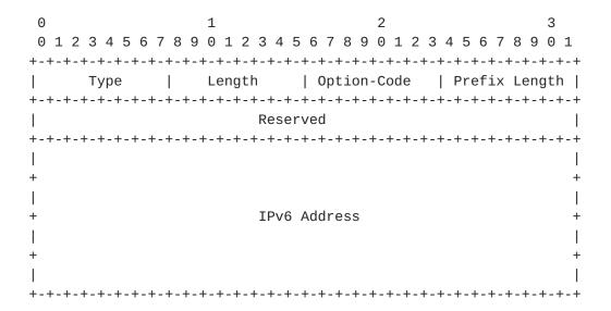
Figure 12: IPv6 Address Option
