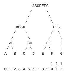
Each node in the tree is assigned a \_node index\_, starting at zero and running from left to right. A node is a leaf node if and only if it has an even index. The node indices for the nodes in the above tree are as follows:
