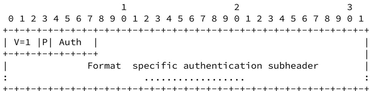
Figure 3: Format of the authentication header
