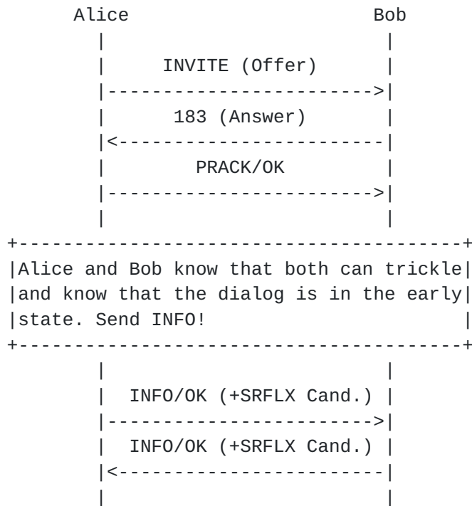
Figure 3: SIP Offerer can freely trickle as soon as it receives an Answer.
