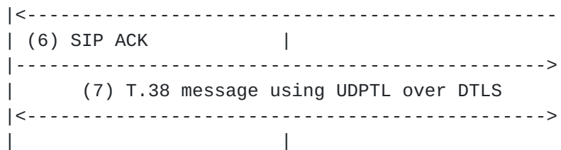
Figure 6: Message Flow Of T.38 Fax Replacing Audio Media Stream in An Existing Audio-Only Session
