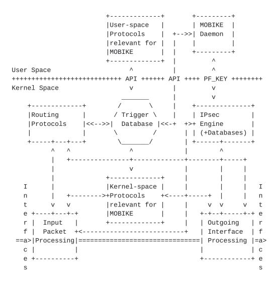
===> = IP packets arriving/leaving a MOBIKE node <-> = control and configuration operations
