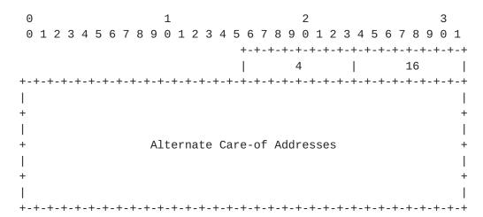
The Alternate Care-of Address sub-option is valid only in Binding Update destination options. The Alternate Care-of Address field contains an address to use as the care-of address for the binding, rather than using the Source Address of the packet as the care-of address.
